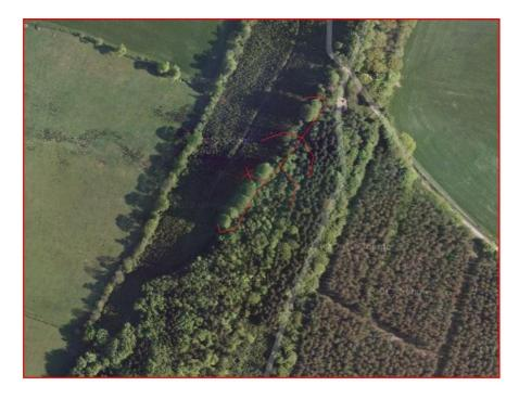
The ridge was covered in thick vegetation with plenty of trees to hold up the antenna system. Several dummy quarter wave, earth staked antennas criss-crossed the main long wire radiating element.
