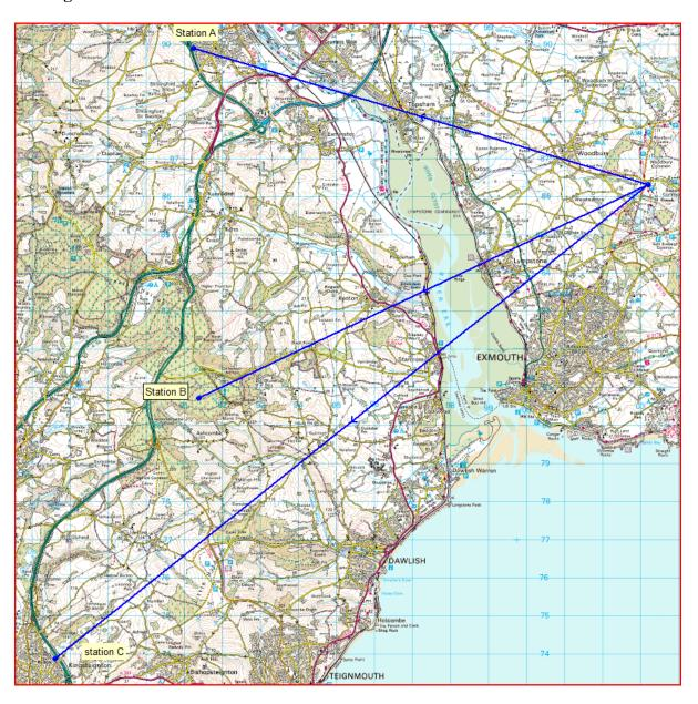
A bearing 283deg @ 12.4km, B bearing of 240deg @ 13km and C bearing 228deg @19.9km.
